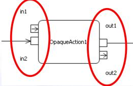
Expansion node: provides inputs and outputs to an expansion region.
